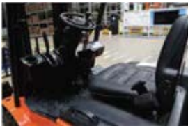
Combination switch as automotive, the seat can be adjusted back and forth so that the operator can choose the ideal driving position.
