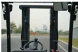
Wide view through the optimized mast and hydraulic design, the forks with intelligent buffer, protect the ground and goods from damage from hitting the ground.
