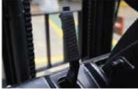
The truck adopts long tiller ratchet parking brake design for easy operation.
