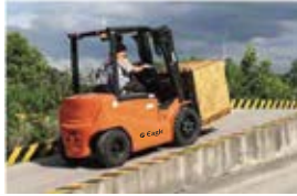
Ratchet-type parking brake allows the truck stay at the slope of 15% without safety concern.
